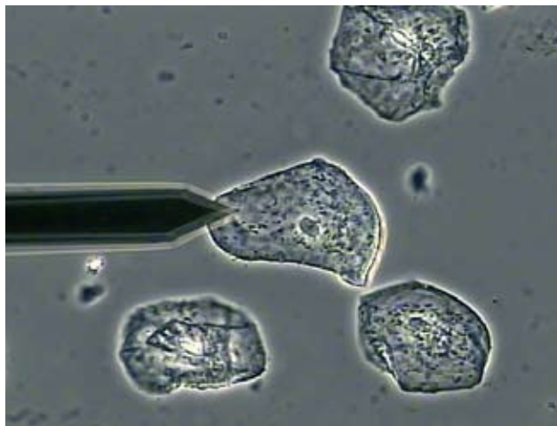
Phase contrast optical micrograph of epithelial cell and AC240 cantilever. Imaged with an Olympus LCAch 20x/0.40 PhC objective.
